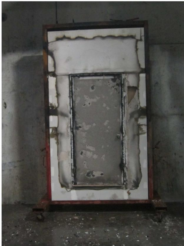
Exposed Side After the Hose Stream Test
