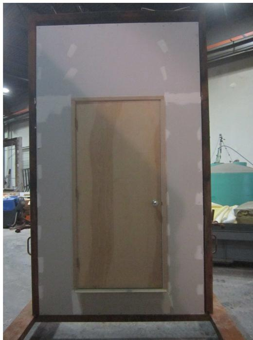
Exposed Side Prior to the Fire Test
